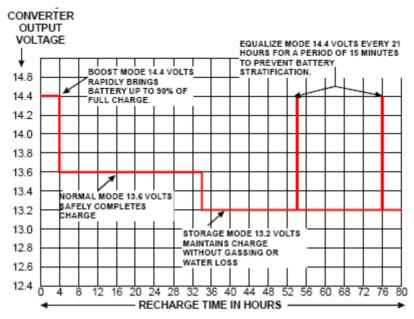
**14.4 Volts (Boost Mode)** Rapidly brings the batteries up to 90% of full charge / LED is steady ON
